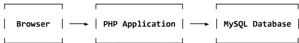
Figure 2.1 High-level system architecture
